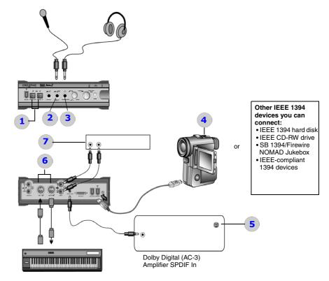
Figure 2-8: Connecting peripherals to the External I/O Module.
